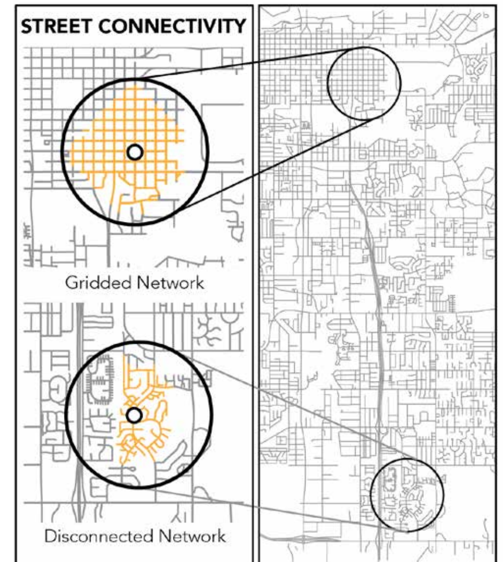
Figure 39: In a connected street network, as in downtown Anchorage (inset at top), nearly all of the places within 1/2 mile of a transit stop are within a 1/2 mile walking distance. In a disconnected network, as at bottom, a transit stop might be within 1/2 mile of many activities by flying distance, but the lack of street connections means that few people nearby the stop can actually access it by walking less than 1/2 mile.
