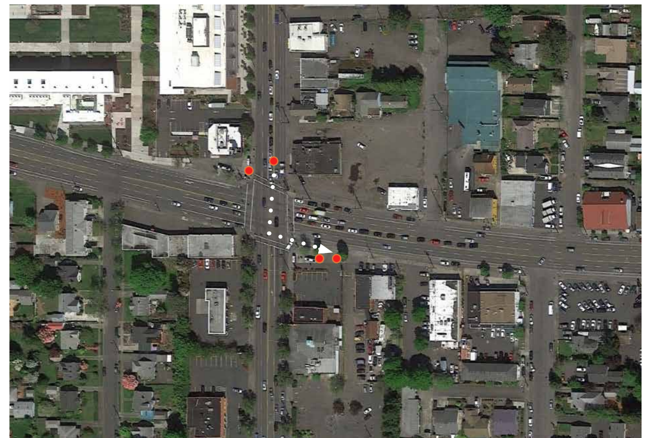
Figure 44: At left, bus stops are not allowed near the intersection of Lake Otis and Tudor, so transferring between routes there can involve a 1,000 foot walk (about 1/8 mile). In addition, people walking between bus stops face long waits to cross the street, and frightening crossings of right-turn slip lanes that are uncontrolled by traffic lights. At right, a pair of large roads in East Portland intersect. Both are served by frequent buses, and the bus stops have been placed as close to the corners as possible, allowing people to transfer with short walks or, for some directions, no walk at all.
