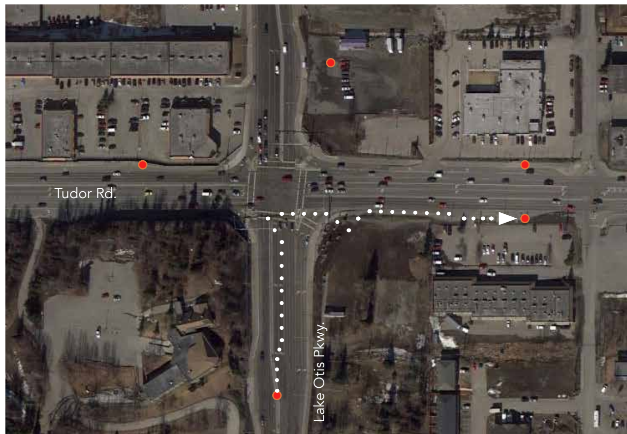
Figure 44: At left, bus stops are not allowed near the intersection of Lake Otis and Tudor, so transferring between routes there can involve a 1,000 foot walk (about 1/8 mile). In addition, people walking between bus stops face long waits to cross the street, and frightening crossings of right-turn slip lanes that are uncontrolled by traffic lights. At right, a pair of large roads in East Portland intersect. Both are served by frequent buses, and the bus stops have been placed as close to the corners as possible, allowing people to transfer with short walks or, for some directions, no walk at all.
