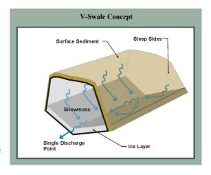
ice headward along the trough of the swale. As removal of the basal ice progressed up the trough, snow pad soils became exposed to erosion and are believed to have contributed to turbidity measured in meltwater at this site. However, exposed trough soils rapidly self-armored, limiting these effects.
