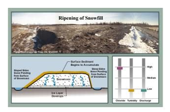
also seems reasonable, given that saturation and beginning of any lateral flow (that might support a localized increase in ice thickness) will not occur until the core snowfill temperatures have risen above those that will support refreezing and formation of basal ice.
