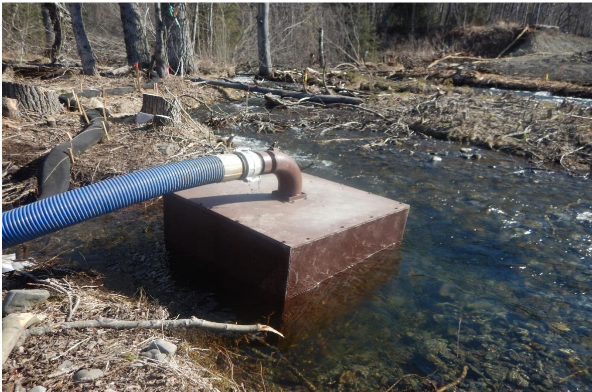
Figure 11. A properly sized intake screen on an intake hose in Indian Creek.
