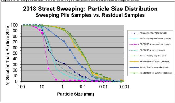
Figure 3-1 Representative PSD of Swept Materials and Residual Samples 2018
