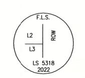
5/8" x 30" Rebar with 2" Aluminum Cap
