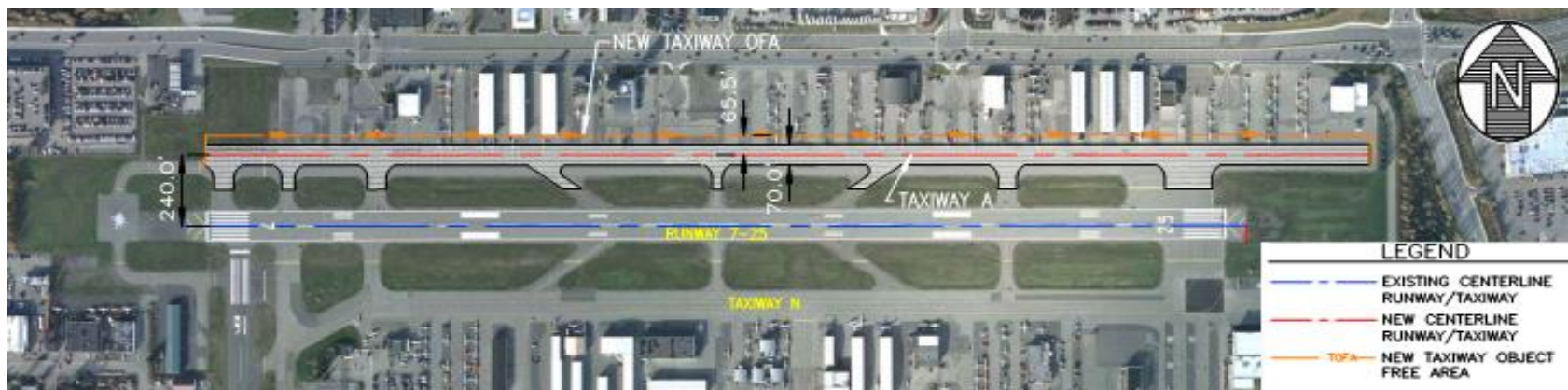
Figure 6-8 Increase Separation between Runway 7/25 and Taxiway A, Option A
