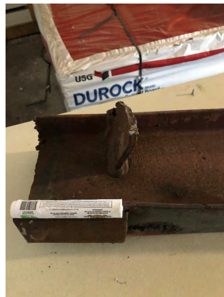
Figure 4.44. (a) Girdwood Wastewater Treatment Facility operations building with a sheared steel crane beam not connected at one end (photo: AWWU); (b,c) Hilton Anchorage steel soffit-beam failure (photo: PND Engineers).
