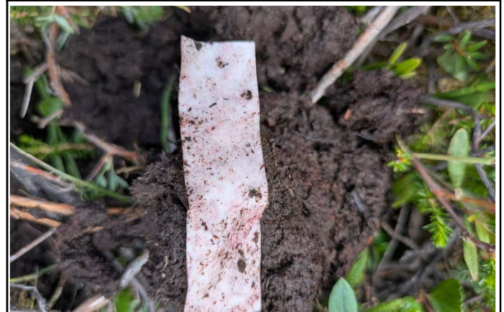
SP1—presence of 'C4—Reduced Iron' using dipyrldyl paper
