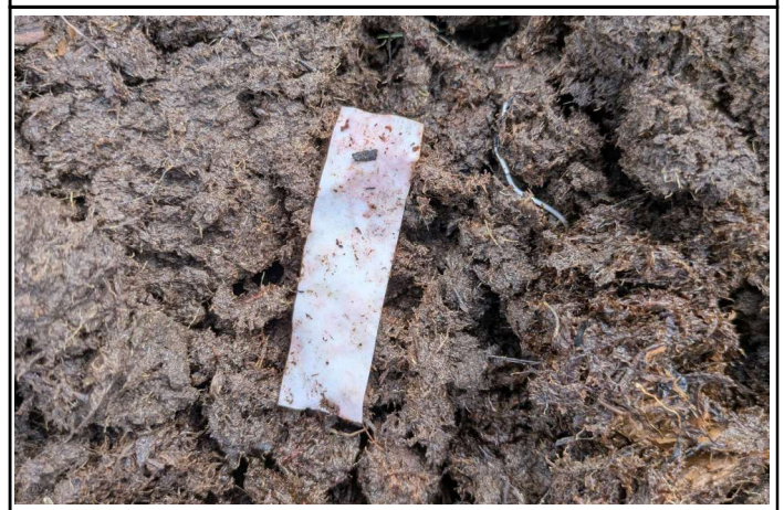
SP2—presence of 'C4—Reduced Iron' using dipyrldyl paper
