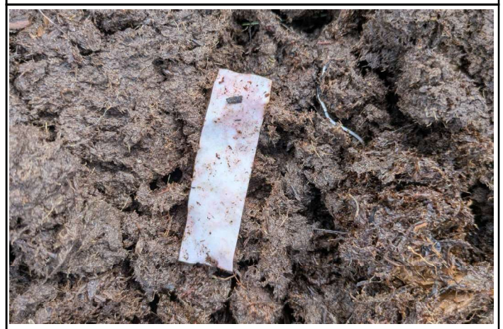
SP2—presence of 'C4—Reduced Iron' using dipyrldyl paper
