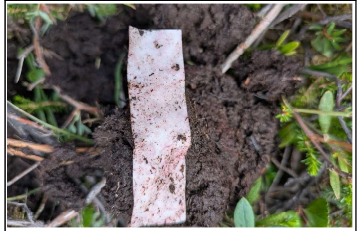
SP1—presence of 'C4—Reduced Iron' using dipyrldyl paper
