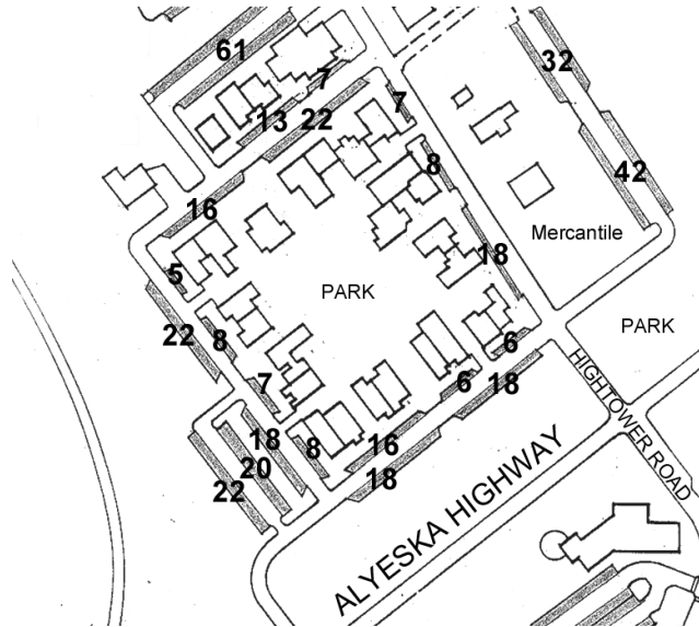
Fig. 7-4 New Townsite parking improvements. Numbers indicate parking spaces added on-street and in public lots to the east and west
