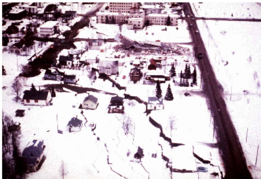
Photo 1.3 A graben formed at the head of the L Street landslide in Anchorage during the earthquake. The slide block, which is virtually unbroken ground to the left of the graben, moved to the left. The subsidence trough sank 7 to 10 feet in response to 11 feet of horizontal movement of the slide block. The volume of the trough is theoretically equal to the volume of the void created at the head of the slide by movement of the slide block. A number of houses seen in this photograph were undercut or tilted by subsidence of the graben. Source USGS.
