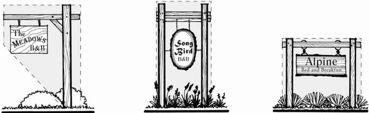
Framing area, defined by the combined outer limits of the sign and all frames and supports.
