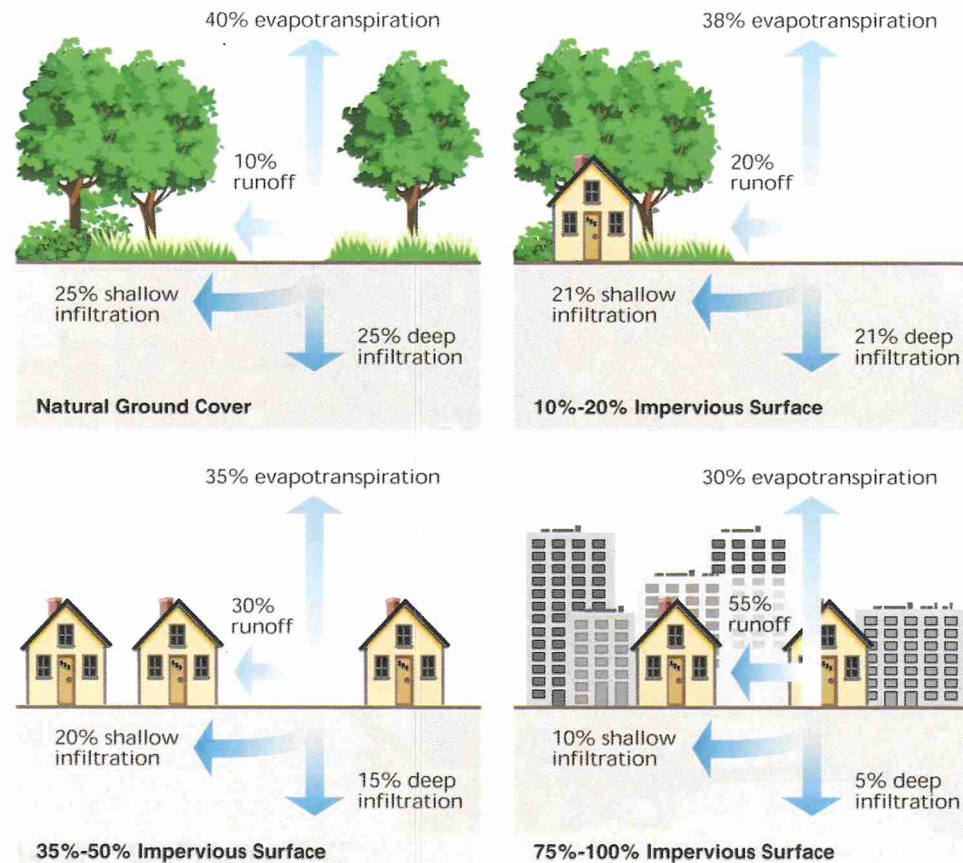
Figure 3.21. Illustration of the Effect of Increased Urbanization on Impervious Surfaces and Surface Runoff 59
