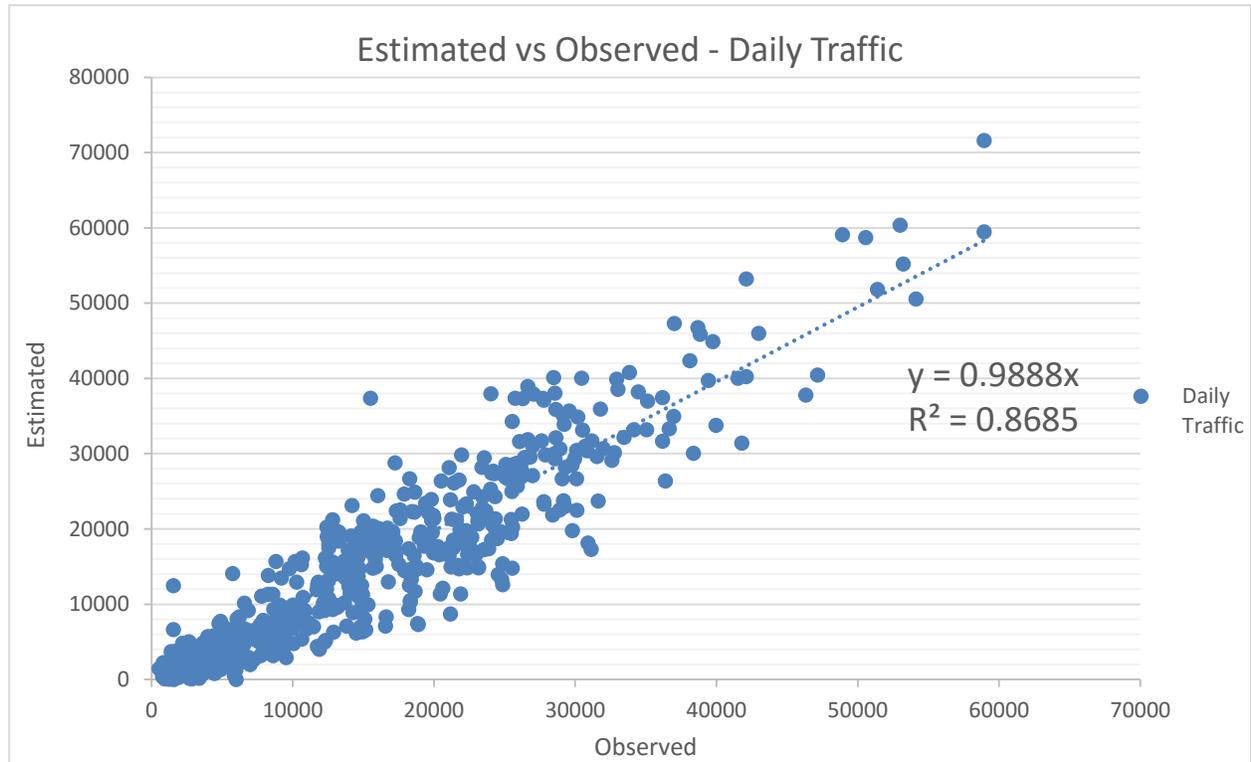
Table 77 shows estimated versus observed daily traffic by observed volume range. Percent root mean square error (RMSE) is a useful statistic that measures the average deviation from counts across all links. The equation for RMSE is given below.
