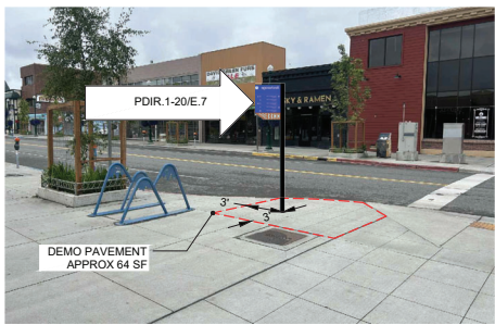
2 SIGN 20 DEMO & INSTALL LOCATION - PDIR. 1 (NORTHEAST CORNER OF W 4TH AVE & E ST)
