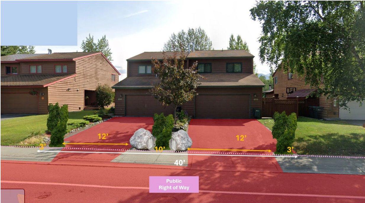
Figure 2 Boulders or other vertical separation may be used to separate drivable surface from the ROW line.
