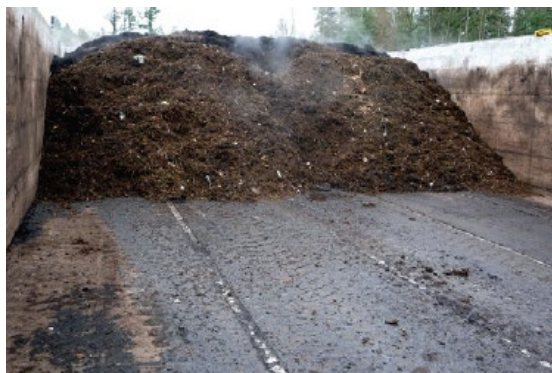
Figure 3-7: Aerated Static Pile Inside Bunker Walls
