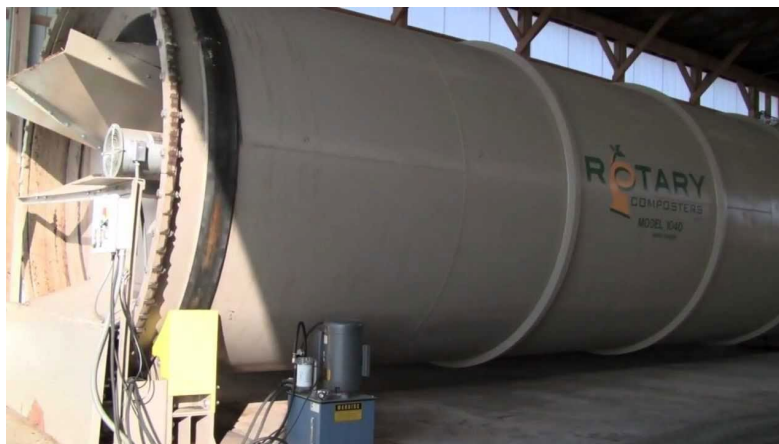
Figure 3-14: Rotating Drum System
