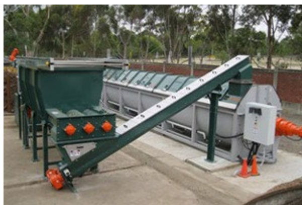
Figure 3-13: Hot Rot Compost System
