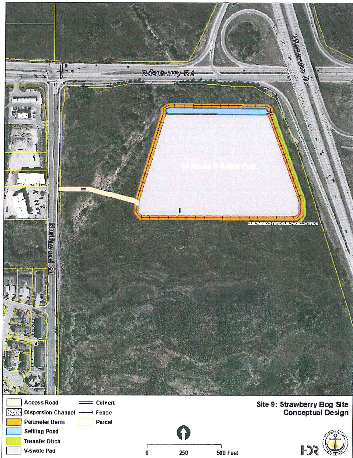
Figure 8. Site 9: Strawberry Bog Site Conceptual Design
