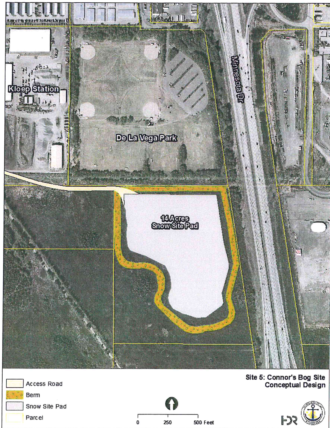
Figure 7. Site 5: Connor's Bog Site Conceptual Design
