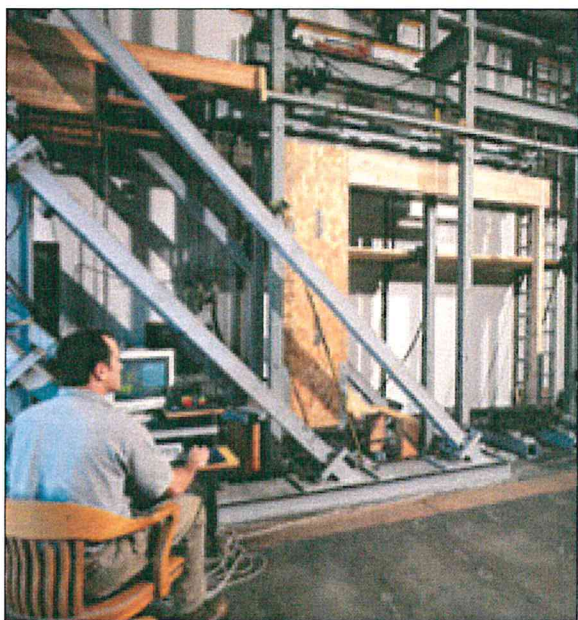
This test in the APA research center simulates seismic lateral loads over dozens of cycles to the same wall line. APA researchers can then determine the suitability of various bracing details for seismic performance, such as extending the glulam header over the narrow end wall.
