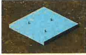
FIGURE 7-9. Concrete base ready for installation
