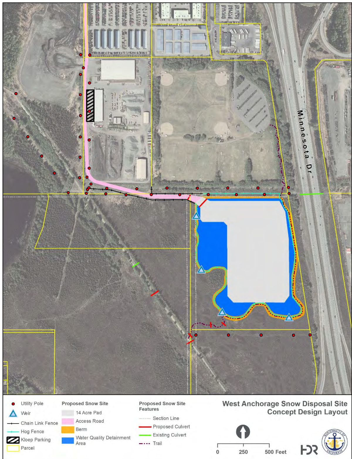
Figure 4 Snow Disposal Pad Conceptual Design Layout
