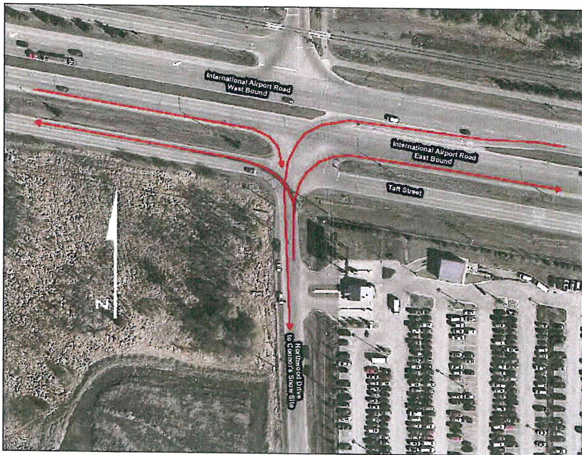
Figure 4. Truck Access to S. Northwood Drive
