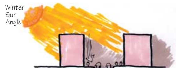
Ineffective Northern Design Technique: Vertical Buildings - Wind drafts effect pedestrian areas - Winter sun doesn't reach the street level
