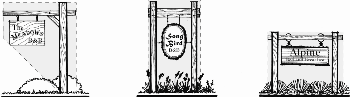
Framing area, defined by the combined outer limits of the sign and all frames and supports.
