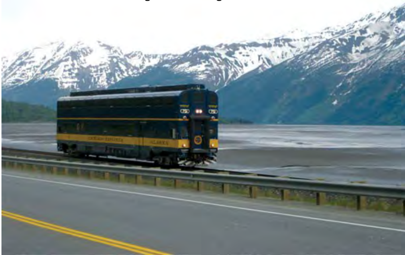
Alaska Railroad's double-deck self-propelled commuter railcar which currently provides whistle stop service at five sites between Portage and Moose Pass
