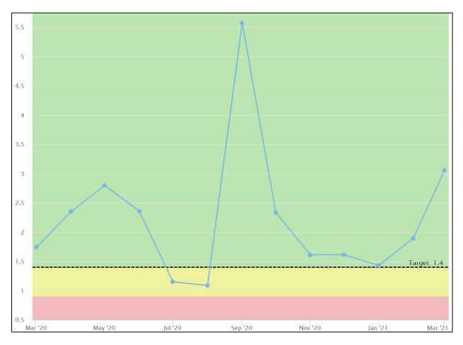
This is calculated by dividing total tons of waste received at the landfill by the total tons of dirt (cover) used, which includes alternative cover.
