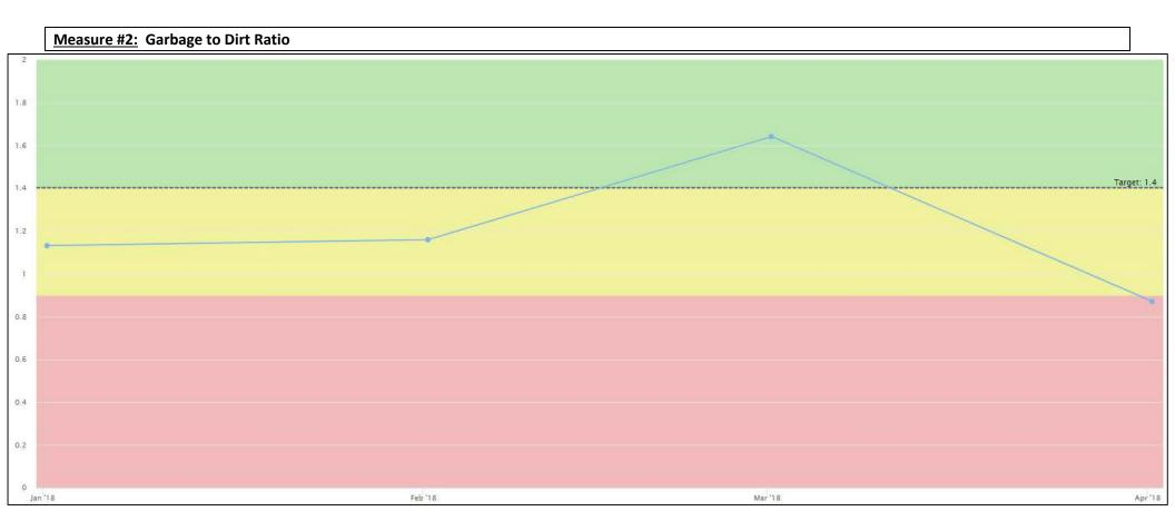
This measure is calculated by dividing the total tons of solid waste received at the landfill by the total tons of dirt used to cover the garbage on a daily basis and displayed as a ratio.
