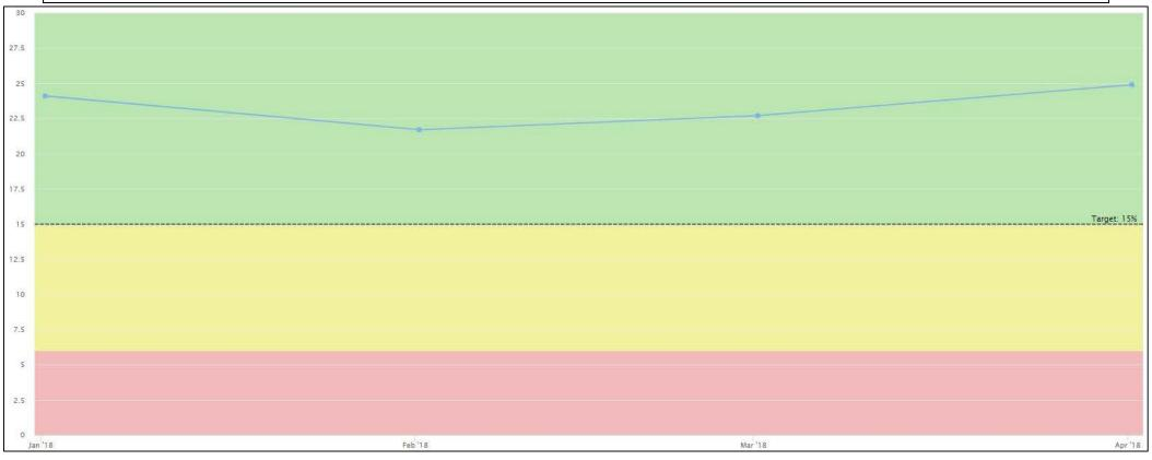
This measure is calculated by dividing the revenue from selling landfill gas by the amount it costs to dispose of waste. SWS has set a target goal of > 15% indicated by the dashed line in the above line graph.
