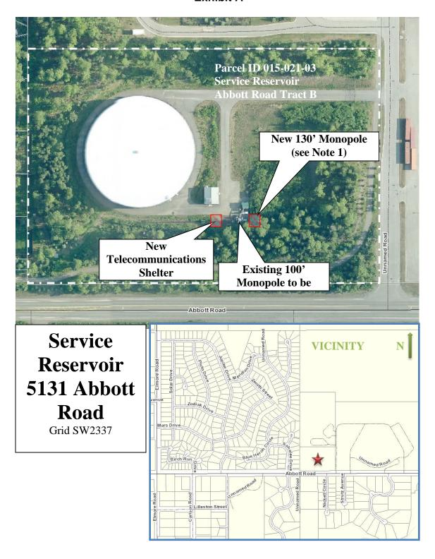
Note1: Existing antennas from existing 100' monopole are to be relocated to the new 130' monopole. A new Verizon antenna is to be installed on the new 130' monopole.
