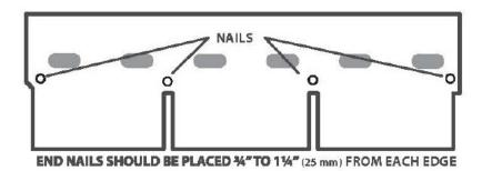
For three tab shingles, fasteners with the minimum of I" long, galvanized roofing nails are recommended by the National Roofing Contractors Association. Nails of I 1/4" long are recommended for ridge shingles and interlocking of dimensional shingles (weaving) as in intersecting planes creating a valley.
