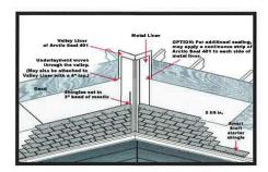
Crop all tops of each shingle course at a 1" (25 mm) 45° cut. Embed the cut valley shingle in a 3" (76 mm) wide bead of mastic (as shown).
