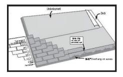
Third Course: Cut 11<sup>1</sup>/<sub>4</sub>" (286 mm) from the left end of the shingle and apply the remaining 281/8" (714 mm) section over the second course shingle, exposing the second course 5\%" (143 mm). Secure with fasteners.
